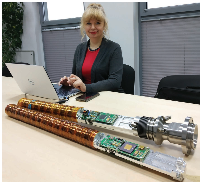
FIGURE 6 – High-precision downhole monitoring system using high-temperature electronics developed by MMB Drives.
