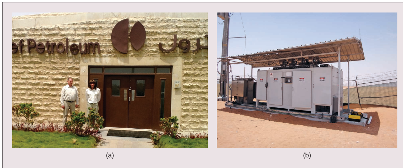
FIGURE 5 – (a) Prof. Krzemiński with his Ph.D. student Janusz Szewczyk at Alkhorayef Petroleum Company, an electric submersible pump (ESP) factory in Saudi Arabia. (b) The world's first power electronic transformer-based, medium-voltage, variable-speed drive with ESP installed on the test rig [1], [9].
